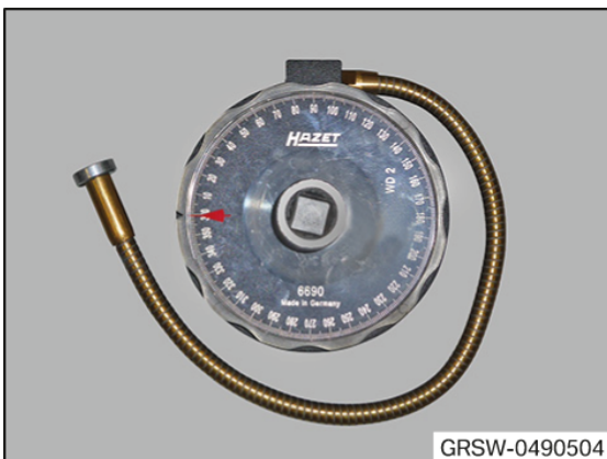
0 490 504 (00 9 120) Torque angle measuring dial
